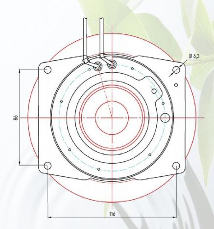
Static break-away torque rating at 12 V DC. Current amp draw is 3.8 A. RES.3.1 $\Omega$  75-85 Lbs.ft.
