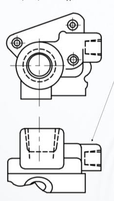
This tank bypass conn. is required for installations which operate at pump relief valve pressures for periods exceeding 15 seconds. Connection must be made below oil level in reservoir.
